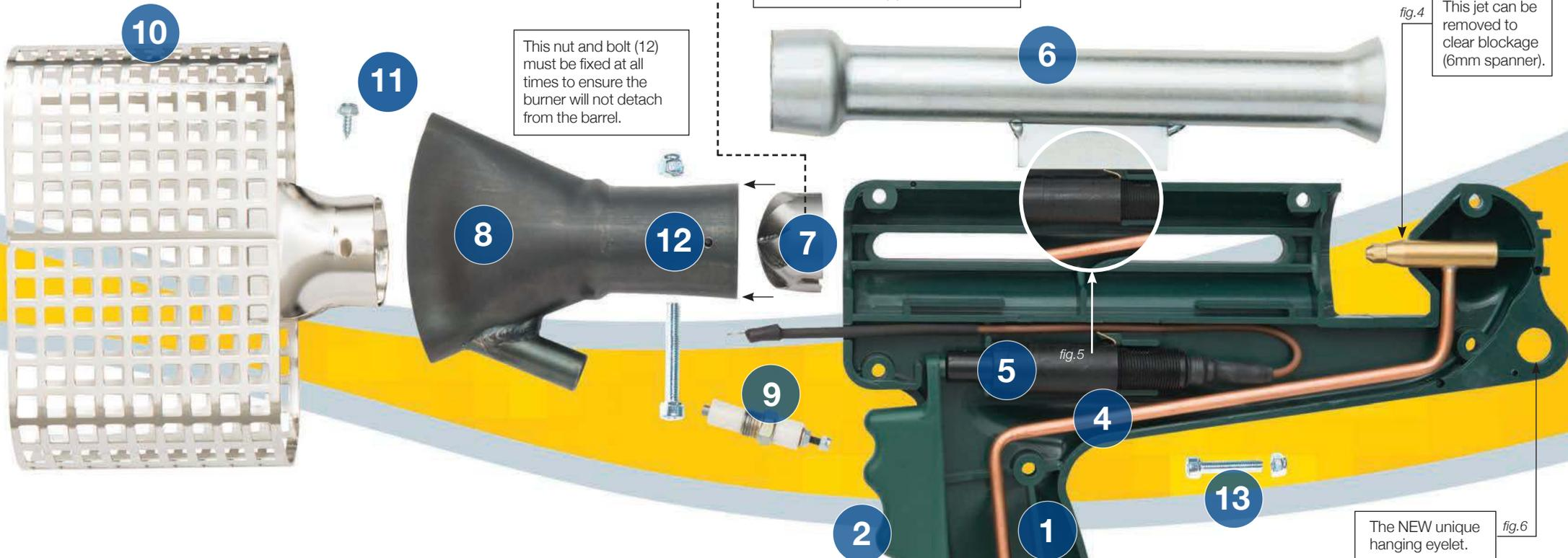
fig.8 Mixer (7) must be fitted a minimum of 19mm into burner (8) as indicated.
